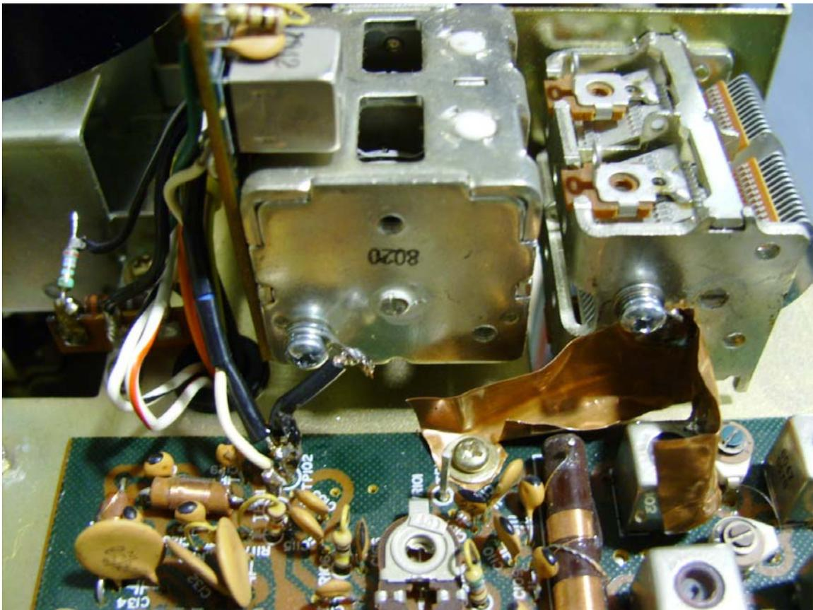
Photo 4. Separate grounds for each tuning capacitor.
