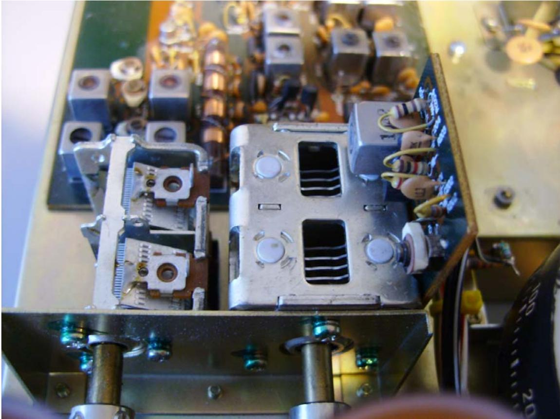
Photo 3. Two tuning capacitors of different systems with a common ground (mounting bracket).
