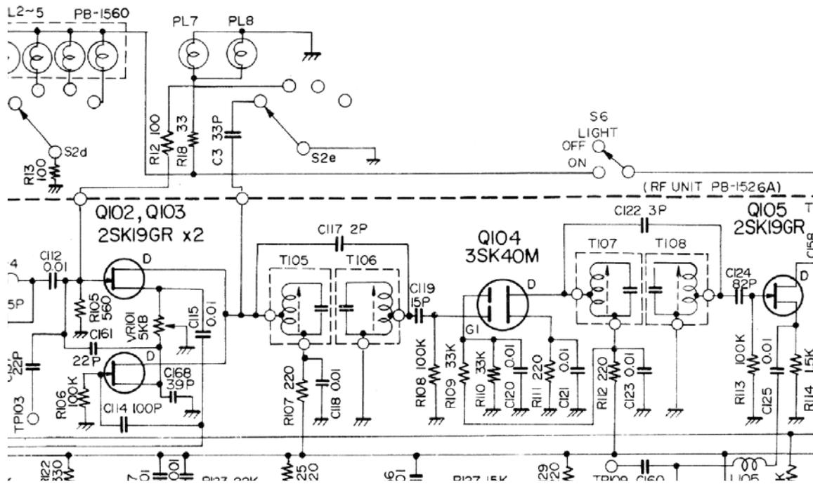
Fig. 2. Part of the schematic diagram of the Yeasu Musen FRG-7 receiver (IF gain switching circuit, with R12 or C3 (RF preselection switch in position A (0.5 – 1.6 MHz) or B (1.6 – 4.0 MHz)).
