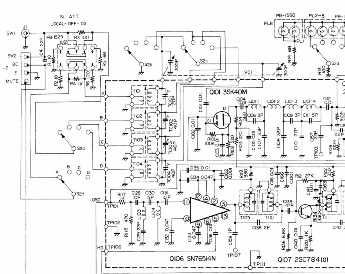
Fig. 1. Part of the schematic diagram of the Yeasu Musen FRG-7 receiver (RF preselection circuit).
