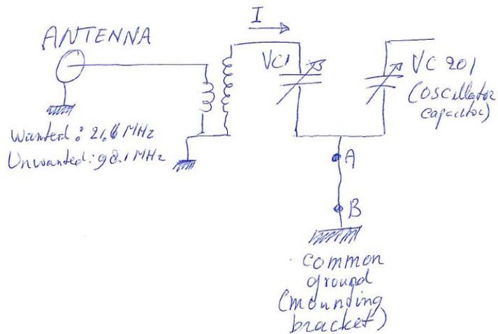
Fig. 4. The schematic diagram of this part of the receiver.
